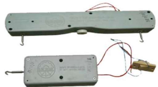
Above: Unit manufactured by Kerala State Coir Machinery Manufacturing Company (KSCMMC) based on CCRI guidelines. KSCMMC's electronic ratt, consisting of a double-spindle part (top), a single-spindle part (bottom-left), and overhead switches (bottom right)
